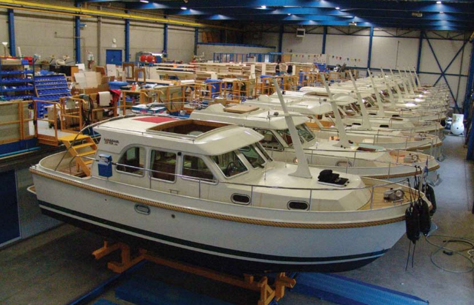
above & below right: the first production line in the world for steel yachts.
