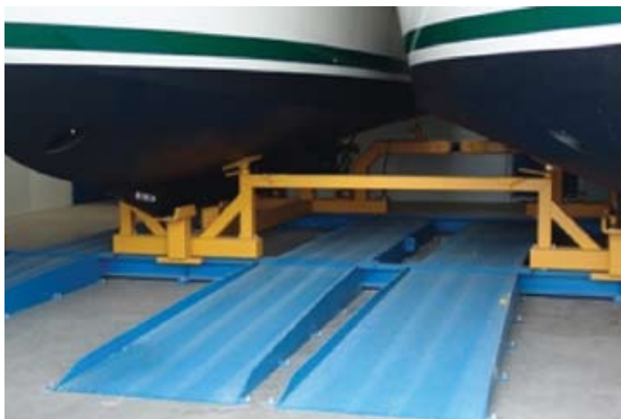
{ 'off ramps' that the totally finished product is rolled off and straight into the water for sea trials}
