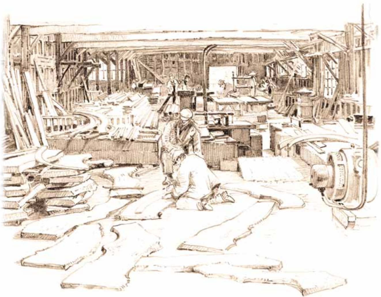
Facing page : Lymington Shipyard Top left : Shaping the stem Top right : Raw materials Below : Setting out the oak frames
