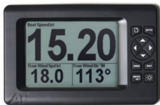
High end display of 'essential' yacht data, in this case from Lymington's A+T Instruments
