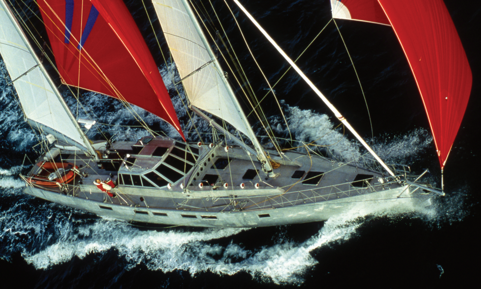
Beowulf with her trade-wind cruising rig. Being an apparent wind machine, she used an articulating bowsprit and full-width travelers for main and mizzen control. She was very well behaved, and only once did we have to cut away a spinnaker.
