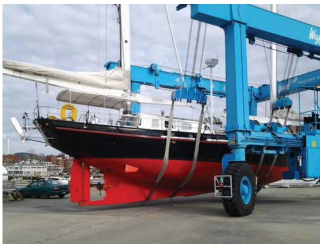
Novara ready for launching. The little fin visible under her quarter is one of a pair of dagger boards which improve tracking downwind when the centreboard is raised
