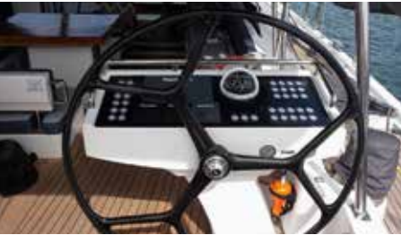
The carbon wheels are original, although the helm station was redesigned and fitted with new Raymarine electronics
