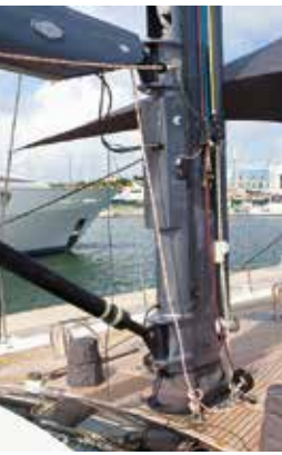
Mast base: the lower third of the mast is original, with the mast rebuilt by Formula Spars
