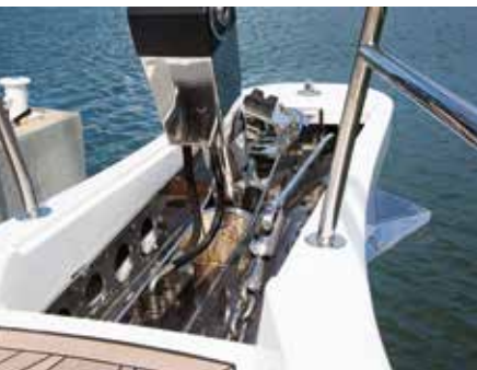
The rebuilt bowsprit complete with 100kg stainless steel anchor
